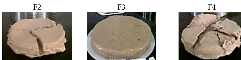
Figure 5. Filter cakes contaminated with salt.
