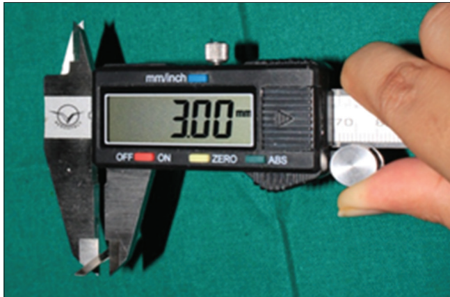
Figure 4: Crosschecking width of casting using digital vernier Caliper
