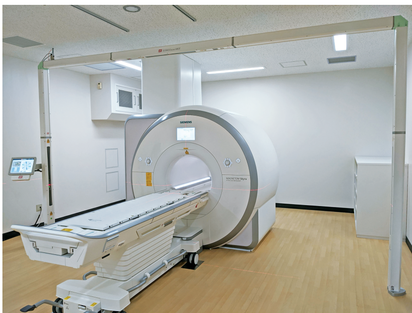
Fig. 1 Dedicated 3T MRI scanner (MAGNETOM Skyra, Siemens, Erlangen, Germany) with an external laser control system (DORADOnova MR3T LAP GmbH Laser Applikationen, Luneburg, Germany) and flat table overlay (Civco Medical Instruments Inc.) placed over a standard receiver coil
