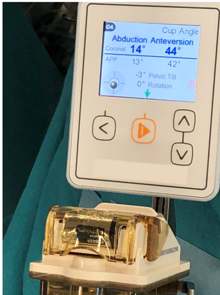
Fig. 1 On the screen of the main unit, inclination and anteversion are displayed in radiographic values during cup insertion and after cup placement. Pelvic tilt and rotation are displayed at any given point in time
