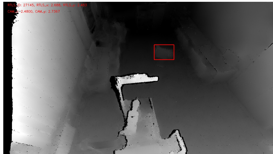
Figure 12. Supply trolley recognition with the help of RTLS and a depth camera. The red rectangle represents an identified object based on depth change, and its location is verified against the RTLS system.
