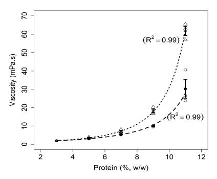
**Figure 2.** Relationship between viscosity and protein concentrations for milk (dashed line) and mixed protein (dotted line) samples. The figure shows the data points for milk (circles) and mixed samples (triangles), error bars (SE), fitted curves, and adjusted coefficients of determination (R<sup>2</sup>).
