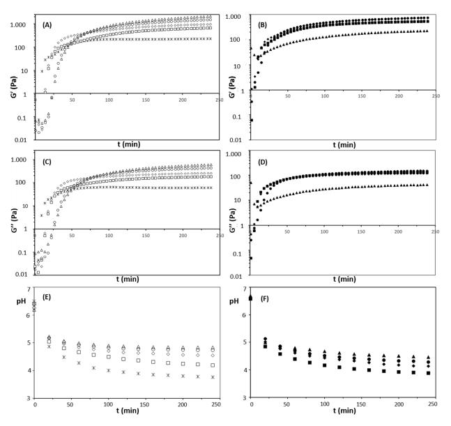
**Figure 7.** Evolution of elastic (G') (**A**,**B**) and viscous shear moduli (G'') (**C**,**D**), and pH (**E**,**F**) as a function of acidification time (t) for milk (open symbols) and mixed suspensions (closed symbols). The square, diamond, circle, and triangle markers represent 5, 7, 9, and 11% (w/w) protein, respectively. The control milk sample is represented by the "x" symbol.
