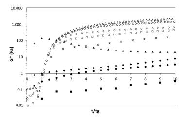
**Figure 6.** The evolution of the complex shear modulus ( $G^*$ ) as a function of reduced time (t/tg) for milk (open symbols) and mixed suspensions (closed symbols). The square, diamond, circle, and triangle markers represent the 5, 7, 9, and 11% (w/w) protein concentrations, respectively. The control milk sample is represented by the "x" symbol.
