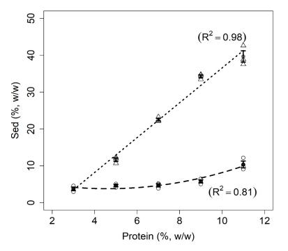
**Figure 4.** Relationship between sedimentable material (Sed % w/w) and protein concentrations for milk (dashed line) and mixed protein (dotted line) samples. The figure shows the data points for milk (circles) and mixed samples (triangles), error bars (SE), fitted curves, and adjusted coefficients of determination ( $\mathbb{R}^2$ ).
