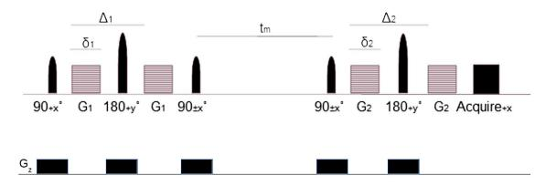
**FIGURE 1** The pulse sequence used in DEXSY,  $G_z$  Slice encoding gradient, diffusion-encoding gradient strength,  $G_1$ ,  $G_2$ , the mixing time,  $t_m$ , the duration of the diffusion encoding gradients  $\delta_1$ ,  $\delta_2$ , and the diffusion times  $\Delta_1$ ,  $\Delta_2$
