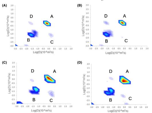
**FIGURE 5** DEXSY diffusion-diffusion plots calculated from in-vitro measurements in yeast, at baseline (t = 0) in sample 1 (A), and at t = 102 min (B). The same plots are shown from sample 2 at baseline (C) and at t = 102 min (D). Sample 1 contained a lower concentration of yeast (18 g in 10 mL PBS) than sample 2 (22 g in 10 mL PBS). Peaks A-D are labeled according to the convention defined above
