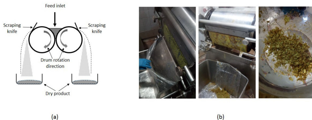
Figure 1. Double-drum dryer (a) operation scheme and (b) operation images.
