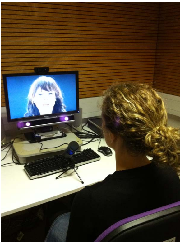
Figure 1. Image of the experimental setup. Participants sat in front of a widescreen monitor, which could display either pre-recorded videos or a live video-feed of an experimenter in a separate room. A webcam was installed above the monitor and a desktop eyetracker sat below the monitor. A microphone was placed in front of the participant. The experimenter sat in front of an identical setup in a separate room, but without an eyetracker.
