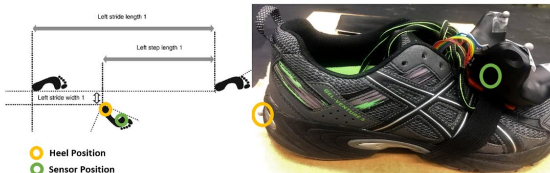
**Figure 3.** Schematic SL and SW from walkway [31]: position of the VR tracker on the foot upper back (green) and heel position (yellow) used for said features calculations.
