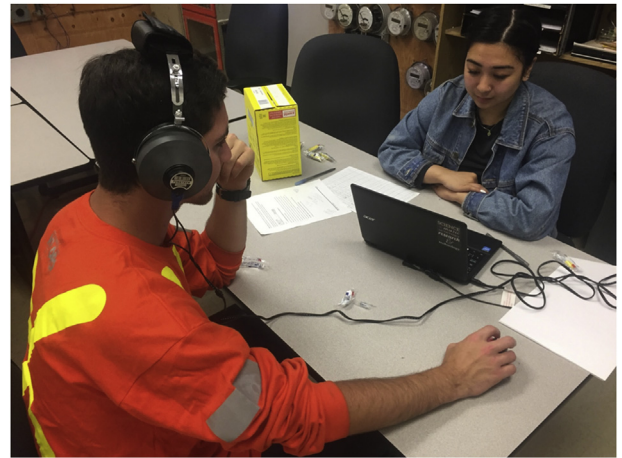
Fig. 1. FitCheck Solo procedure. The experimenter sits facing the laptop and uses the laptop touchpad to progress through the experiment. The participant wears circumaural headphones to hear the stimuli and selects the threshold levels using a computer mouse. A new pair of HPDs is used after each occluded measurement. HPD, hearing protection device.
