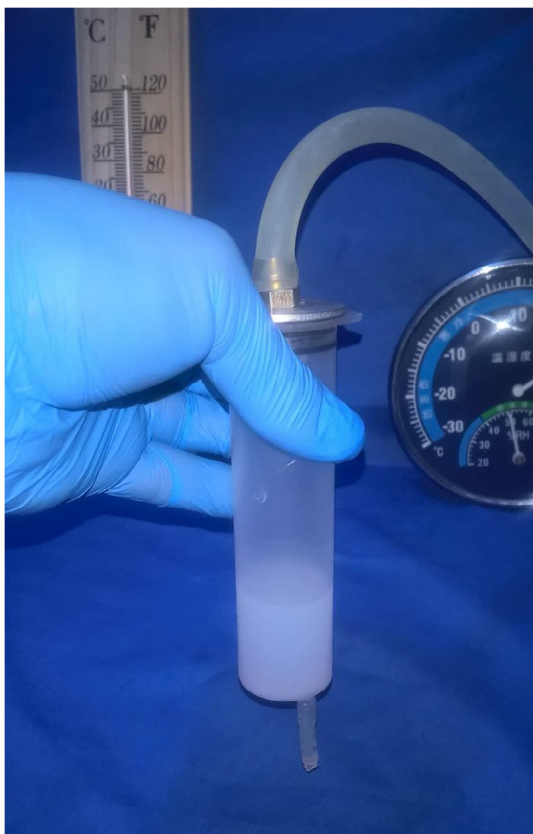
Fig. 1 Deaeration of silicone in the syringe after mixing with the catalyst.
