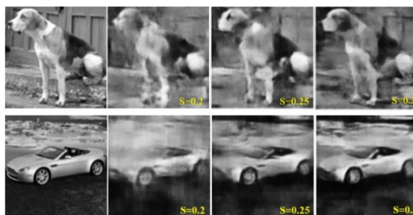
Figure 11. Improving image quality by increasing sampling ratio ( S=0.2, 0.25, and 0.3 ).
