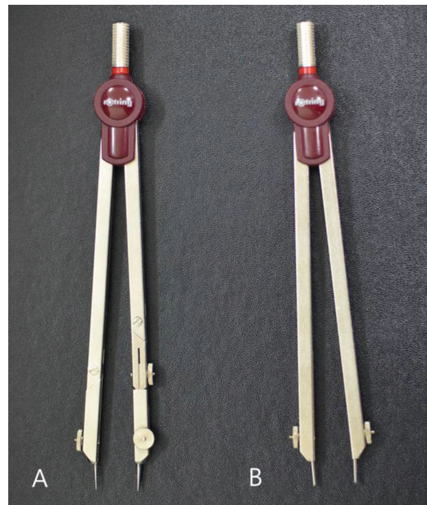
A; drawing compass with sharp-pointed tip B; drawing compass with blunt-pointed tip
