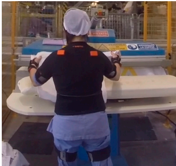
Figure 1. Placement of inertial sensors on a worker. Sensors are the orange probes, when visible, or inside the black belt.
