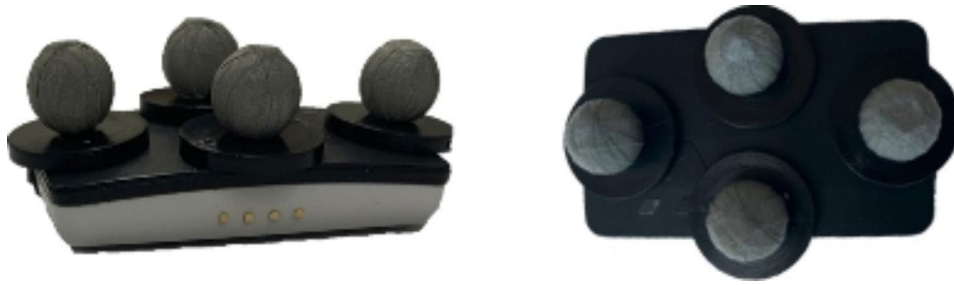
Fig. 1 The DorsaVi Version 6 sensor with Vicon markers placed on top (side and top view)
