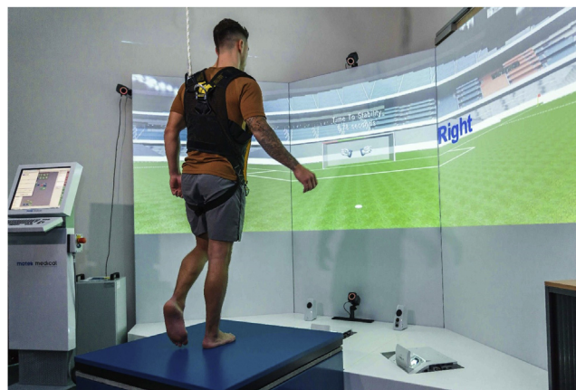
Figure 1. The set-up of the position-controlled movable platform with an integrated force plate and the screen providing real-time visual feedback.
