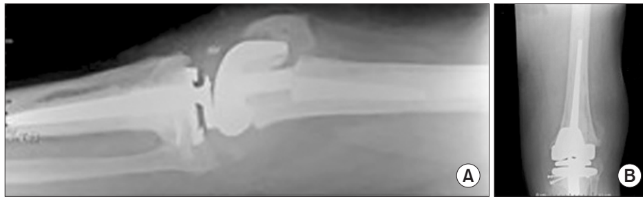
Fig. 3. Radiographs of case 3. (A) The femoral stem is fractured at the point where its diameter changes. (B) There are radiolucent lines around the proximal part of the tibial stem but this was asymptomatic and the tibial component was well fixed at the time of surgery. The femoral component was revised with a longer stemmed component.
