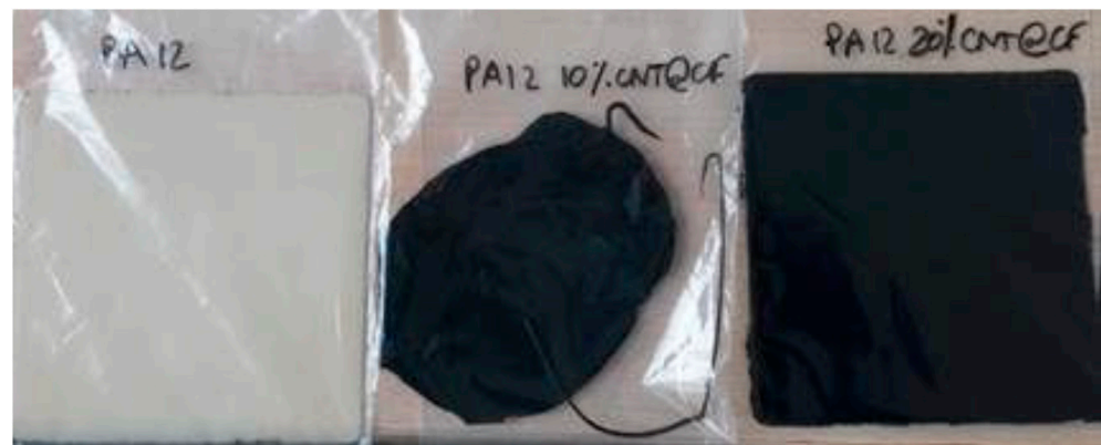
Figure 6. The fabricated coupons of PA12 and PA12 with 10% and 20% inclusions of CNTs@chopped CFs.
