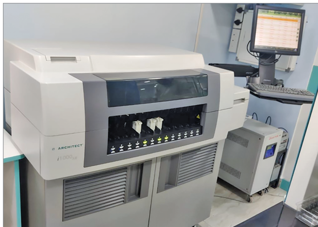
Fig. 2: Abbott Architect c system
