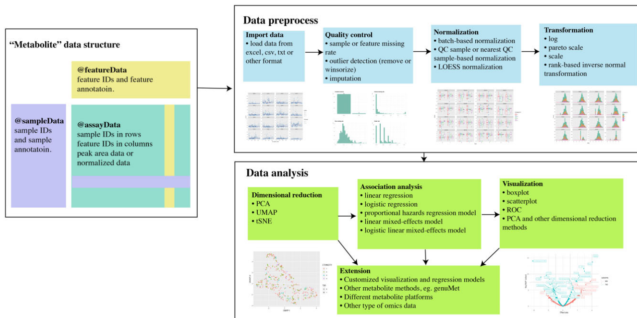
Fig. 1. Streamlined workflow to preprocess, analyze and visualize metabolomics data in metabolomicsR. The main functions are categorized in each box. The sub-panel figures are displayed for illustration. The preprocess step includes procedures for quality control, outlier detection, missing value imputation and transformation, etc.
