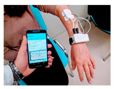
Figure 2. µEMG experimental system: wearable device and mobile app.
