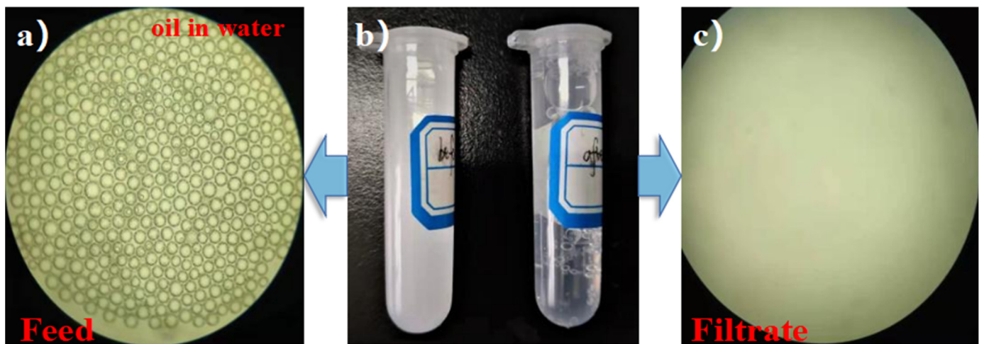
Figure 9. Optical microscope images of petroleum ether/water emulsion, (a) before separation, (b) macro photos of the emulsion before and after separation, (c) after separation.
