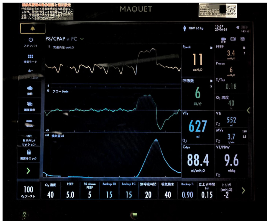
Fig. 3 The ventilator display during the second spontaneous breathing test with pressure triggering. Inspiratory pressure (up), flow (middle), and tidal volume (bottom) waveforms indicate low respiratory rate (6/min) with large tidal volume (627 ml)
