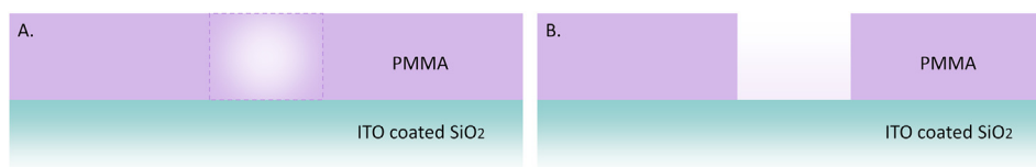
Figure 2. A cross section of PMMA on the ITO/SiO 2 substrate with the (A) active exposed area during exposure, but before development and (B) after exposure, after development.
