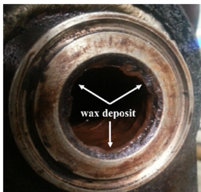
Figure 1. Exhibition of the wax deposit formed in a pipe.
