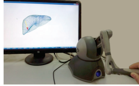
FIGURE 5: Experimental environment based on PHANTOM Omni.
