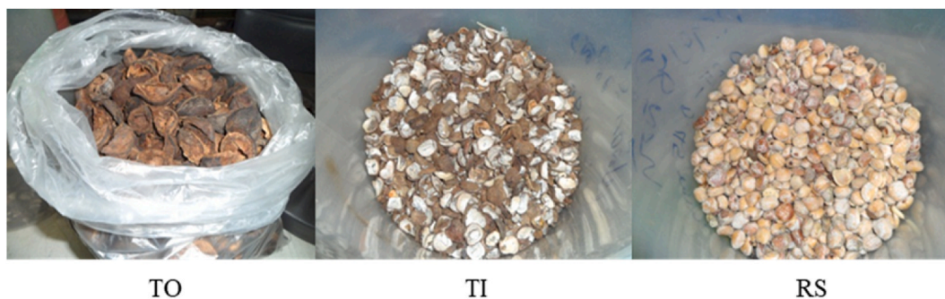
Fig. 2. Three parts of Tung seed residues, Tung seed outer shell (TO), Tung seed inner shell (TI) and the pressed residues of oil seeds (RS).
