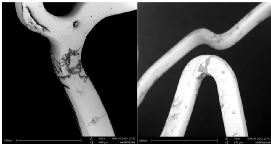
Figure 2. Representative SEM images of EES and PF-SES, magnification \times 350 . Representative SEM images of EES (left panel: EES with fibrin strands) and PF-SES (right panel: PF-SES with some small spots of fibrin), magnification \times 350 . BMS, bare metal stent; EES, everolimus-eluting stent; PF-SES, polymer-free sirolimus-eluting stent; SEM, scanning electron microscopy.
