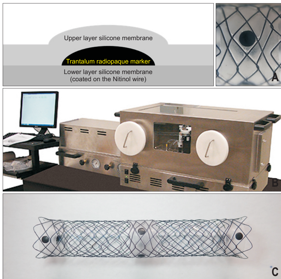
Fig. 1. A novel tantalum marker, the ultrasonic coating machine used, and a Nitinol alloy SEMs with novel tantalum markers. (A) Schematic image of a novel tantalum marker and photograph of a marker on a stent. (B) Ultrasonic spray coating machine (Medi-Coat 2jx, Sono-Tek). (C) Nitinol alloy stent with a novel tantalum marker (NEXENT biliary stent, Next Biomedical).
