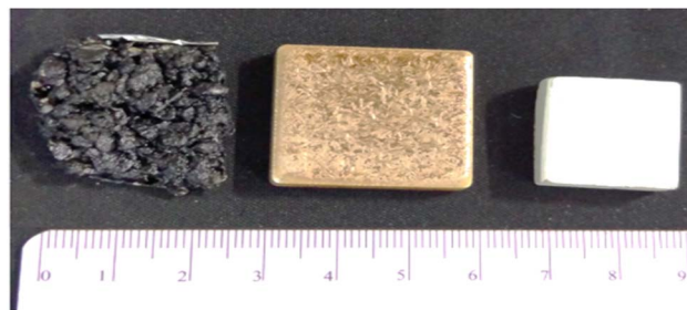
Fig. 1 Photograph of representative material coupons. From left to right, tarmacadam, tile and concrete coupons were cut to size from larger pieces of stock materials and sterilized prior to use in decontamination tests.
