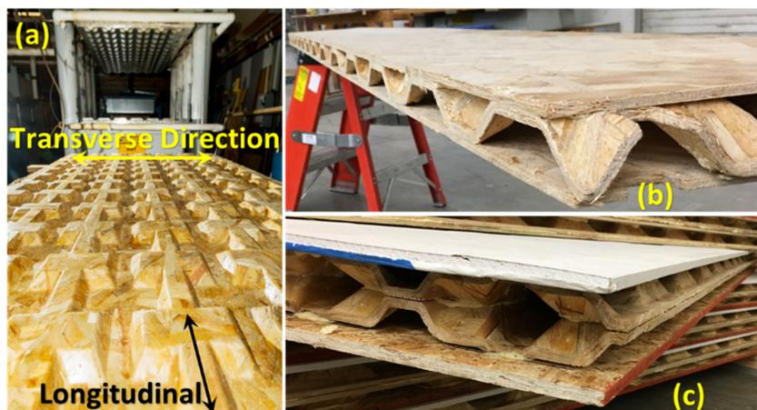
**Figure 1.** (a) Full size biaxial corrugated panel used as a core to fabricate (b) one-layered (c) two-layered core sandwich panels.
