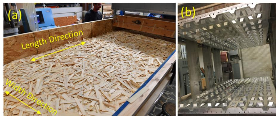
**Figure 3.** (a) Wood-strand mat (*preform*), and (b) Aluminum matched-die mold.
