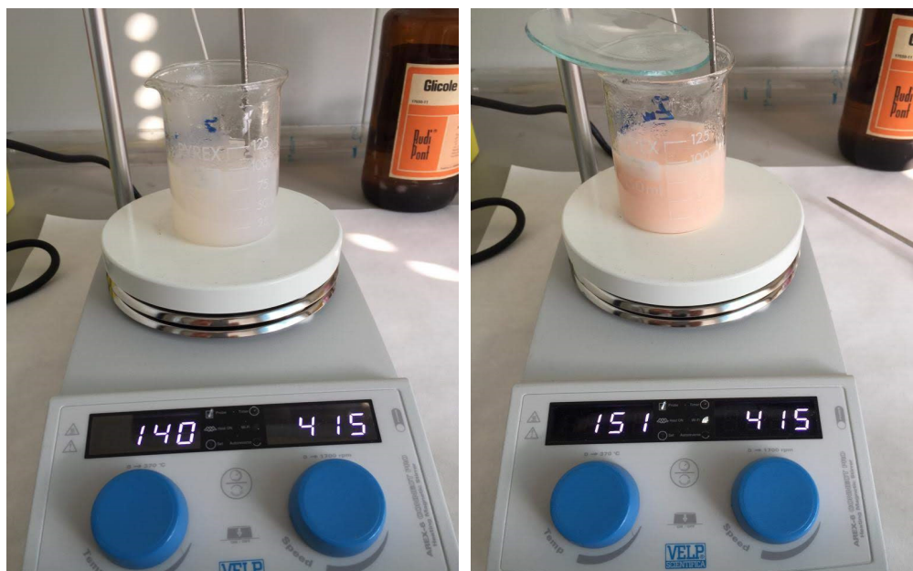
Figure 2. The color of the solution changes with temperature from milky white at 140 °C to rose pink at 150 °C. This change was very quick and easily detectable.
