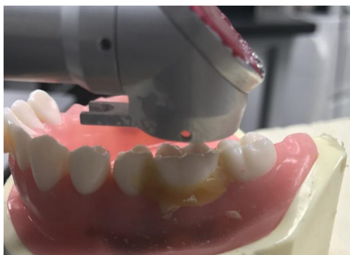
Figure 2. Resin tooth ablated automatically by the dental robot.
