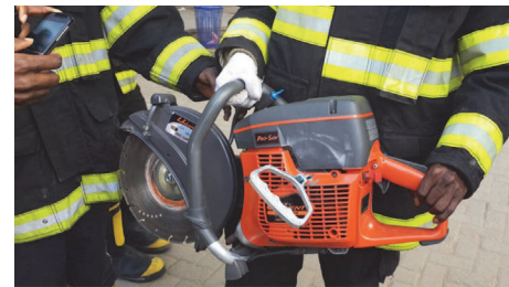
FIGURE 3: Power driven arc saw used by the men of the Lagos State Fire Service.
