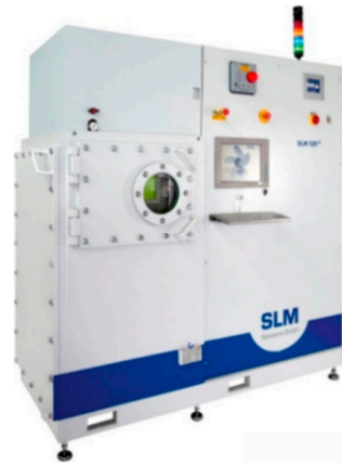
Figure 2. Modified SLM125HL system with overpressure chamber and build chamber reduction to 50 \times 50 \times 50 \text{ mm}^3 .
