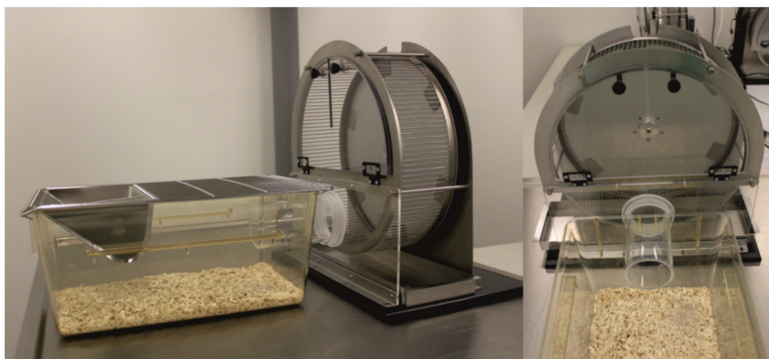
Figure 2. Cages (810 cm 2 ) connected to activity wheels for free-running opportunities during habituation. In the course of experiments, cages were removed and wheels were used for (pseudo-) sleep deprivation.
