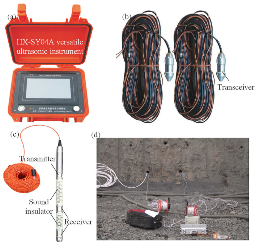
Figure 6. Sonic test system: (a) HX-SY04A versatile ultrasonic instrument; (b) Cross-hole transducer; (c) Single-hole transducer; (d) On-site sonic test.
