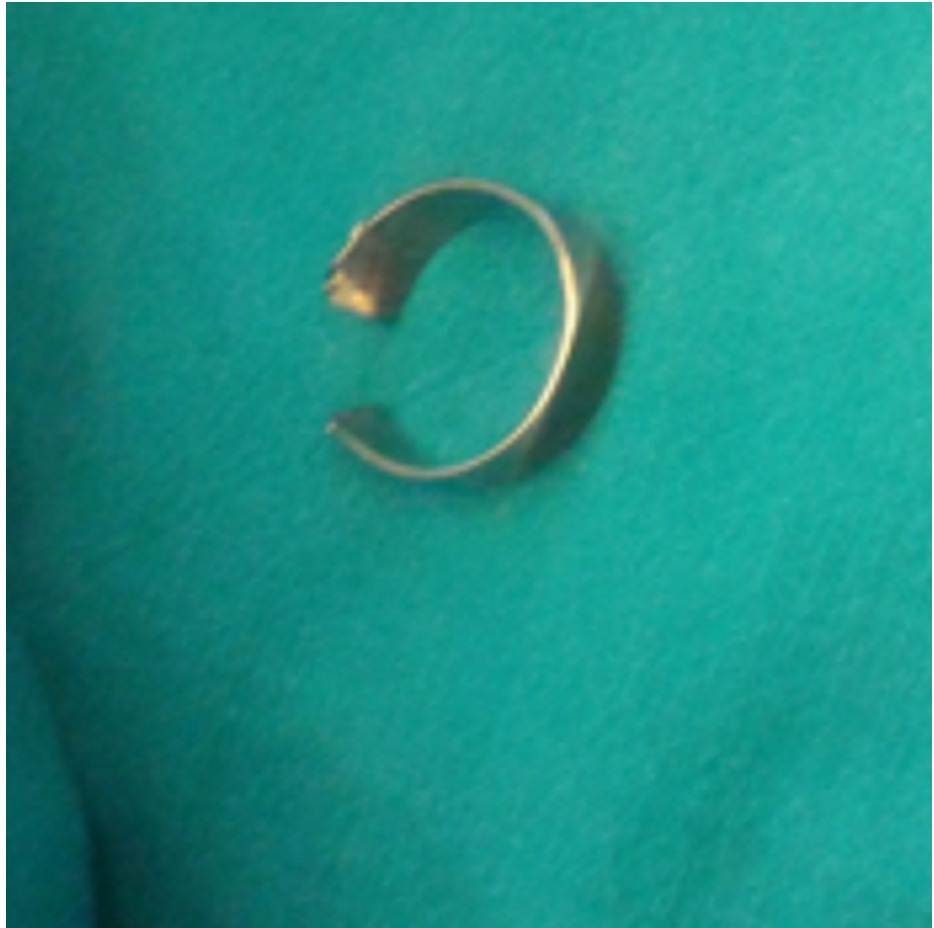
FIGURE 4: Cut ring retrieved after prying the ends open with nose plier.
