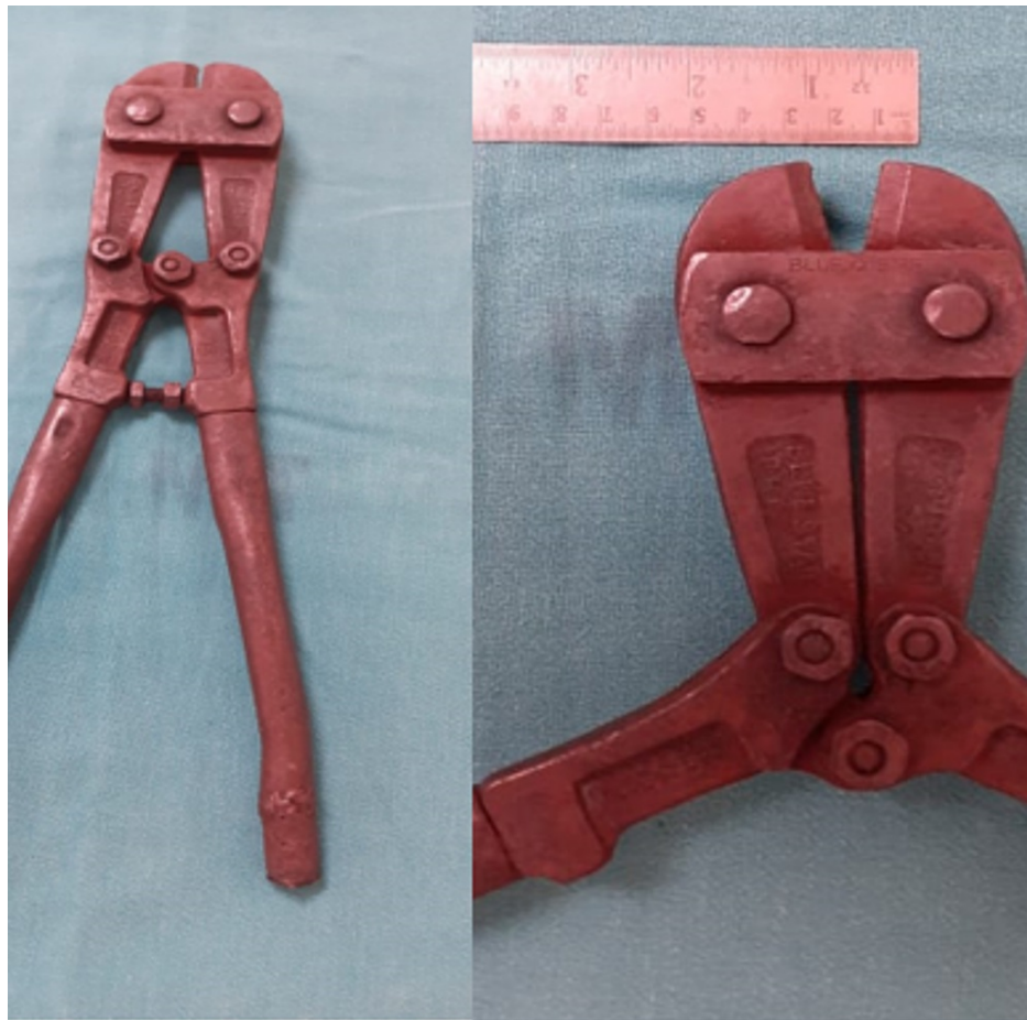
FIGURE 3: Picture on the left - jumbo cutter used to cut the ring. Picture on the right - the jaw of the cutter can open out to 1.5 cm as shown in the image.
