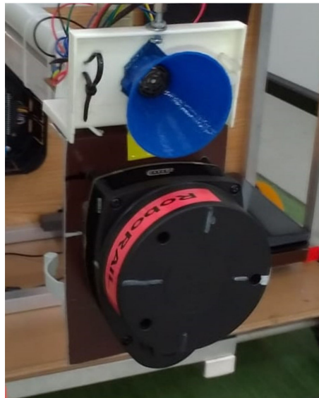
Figure 6. Detail for gauge assessment module with LIDAR scanner and obstacle detection module (ultrasonic).
