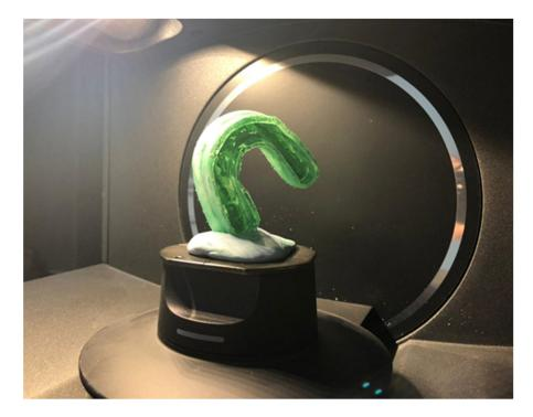
Figure 1. Hybrid mouthguard device positioned in the desktop scanner.
