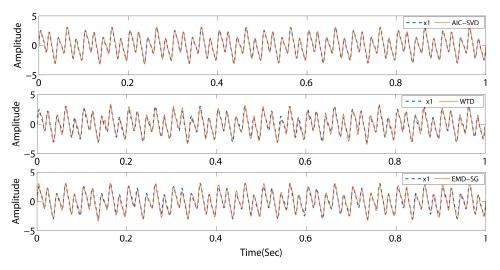
**Figure 5.** Comparison of denoising effects by different methods for signal  $s_1$ . WTD: wavelet threshold denoising; EMD-SG: empirical mode decomposition with Savitzky–Golay filter.
