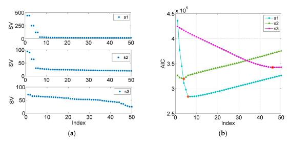
Figure 4. Calculation of simulation signals based on AIC-SVD: (a) singular values; (b) AIC values.
