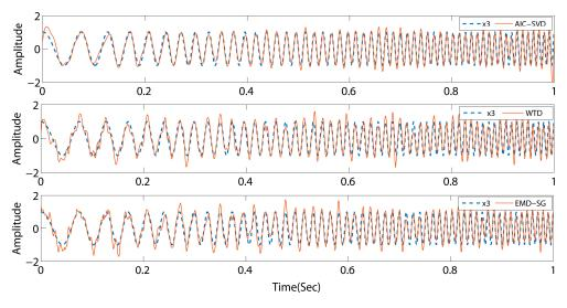
Figure 7. Comparison of denoising effects by different methods for signal s<sub>3</sub>.
