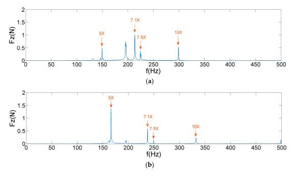
**Figure 16.** AIC–SVD denoised frequency spectra of  $F_z$ : (a) 1800 rpm; (b) 2000 rpm.
