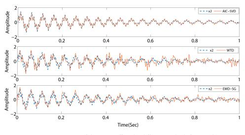
Figure 6. Comparison of denoising effects by different methods for signal *s*<sub>2</sub>.
