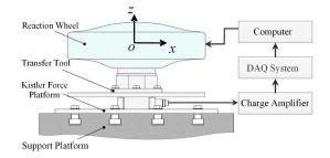
Figure 10. Micro-vibration test of a reaction wheel. DAQ: data acquisition.
