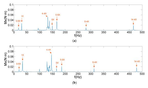
**Figure 17.** AIC–SVD denoised frequency spectra of  $M_x$ : (**a**) 1800 rpm; (**b**) 2000 rpm.
