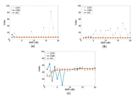
**Figure 1.** Comparison of the different methods in order determination: (**a**) signals  $s_{1(SNRs)}$ ; (**b**) signals  $s_{2(SNRs)}$ ; (**c**) signals  $s_{3(SNRs)}$ . CCR: cumulative contribution rate; CSM: singular value curvature spectrum; AIC: Akaike information criterion; SNR: signal-to-noise ratio.
