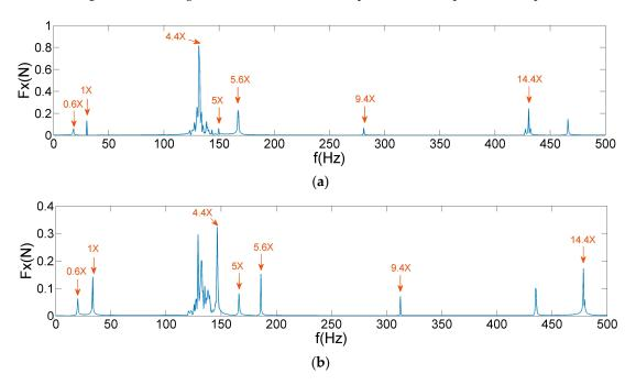
**Figure 15.** AIC–SVD denoised frequency spectrum of  $F_x$ : (a) 1800 rpm; (b) 2000 rpm.
