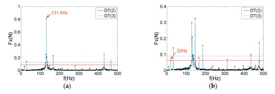
Figure 12. Peak threshold denoising of the micro-vibration signals: (a) 1800 rpm; (b) 2000 rpm.
