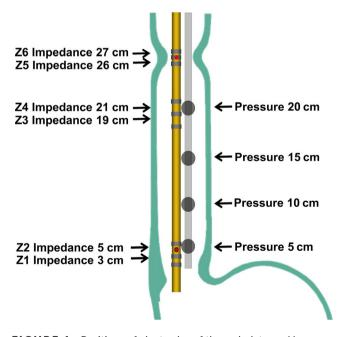
**FIGURE 1** Positions of electrodes of the ambulatory pHimpedance-pressure monitoring system. Red spot: pH electrodes; grey loop: impedance electrodes; black spot: pressure sensors. The values in the figure refer to the distance from the upper border of the lower esophageal sphincter
