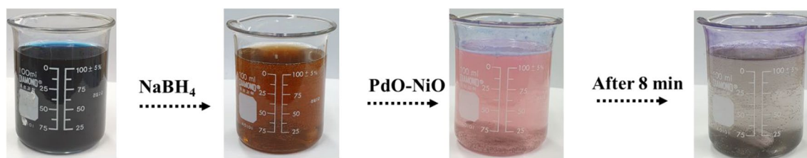
Figure 10. Reaction progress of an azo compounds mixture (4-NP, 2,4-DNP, 2,4,6-TNP, MB, RhB, MO) with PdO–NiO and NaBH 4 . Conditions: Dye: 100 ppm, 25 ml, Nitrophenol: 0.12 mM, 25 ml, NaBH 4 : 0.1 M, 5 ml and catalyst: 3 mg.
