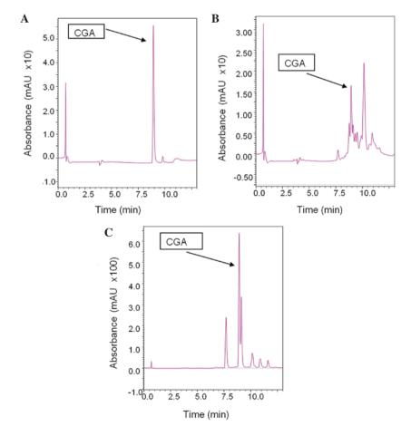
Figure 4. Liquid chromatography (LC)-mass spectrometry (MS) chromatograms of chlorogenic acid (CGA) of (A) standard solution at the concentration of 10 ppm, (B) roasted coffee at the found concentration of 38.8 ppm, and (C) green coffee at the found concentration of 2028.4 ppm.
