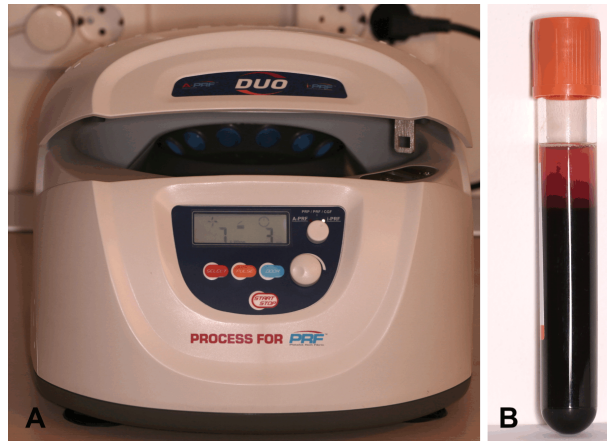
Figure 1 – Preparation of iPRF: (A) Duo Centrifuge; (B) iPRF tube after centrifugation: iPRF is the upper yellow layer. iPRF: Injectable platelet-rich fibrin.
