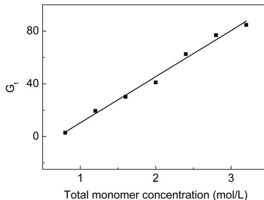
Fig. 2 Variation of  $G_t$  with total monomer concentration. Absorbed dose: 150 kGy; molar ratio of AA to SSS: 1 : 1; reaction temperature: 60 °C; reaction time: 5 h.
