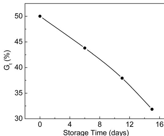
Fig. 5 Variation of  $G_t$  with storage time. Absorbed dose: 150 kGy; molar ratio of AA to SSS: 2 : 1; total monomer concentration: 2 mol L<sup>-1</sup>; reaction time: 2 h.
