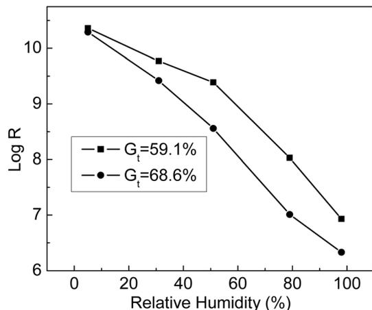
Fig. 11 Relationship between  $\log R$  and relative humidity at different  $G_t$ .
