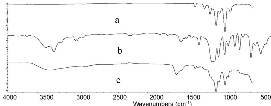
Fig. 6 FTIR spectrum of irradiated ETFE film (a), ETFE-g-AA (b) and ETFE-g-AA-co-SSS (c).
