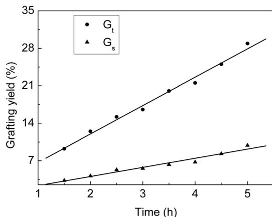
Fig. 1 Variation of  $G_t$  and  $G_s$  with reaction time. Total monomer concentration: 2 mol L<sup>-1</sup>; molar ratio of AA to SSS: 1 : 1; reaction temperature: 60 °C; absorbed dose: 150 kGy.
