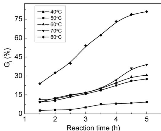
Fig. 3 Variation of  $G_t$  with time at various temperatures. Absorbed dose: 150 kGy; molar ratio of AA to SSS: 1 : 1; total monomer concentration: 2 mol L<sup>-1</sup>.
