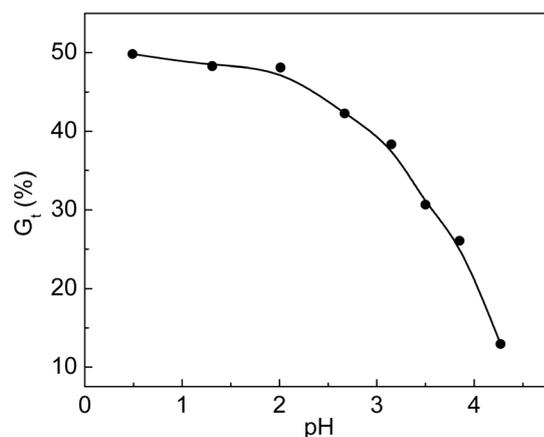
Fig. 4 Variation of  $G_t$  with pH value. Total monomer concentration: 2 mol L<sup>-1</sup>; molar ratio of AA to SSS: 1 : 1; reaction temperature: 60 °C; absorbed dose: 150 kGy; reaction time: 3 h.
