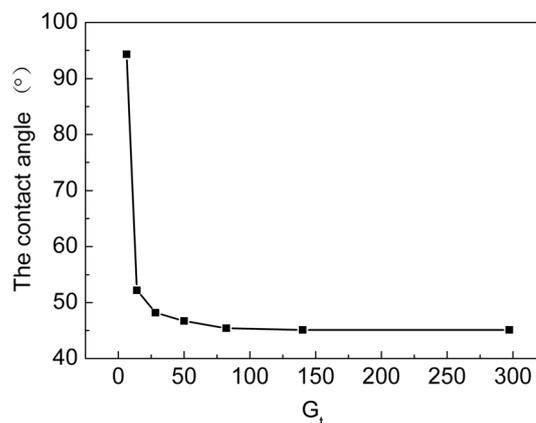
Fig. 8 Relationship between  $G_t$  and water contact angle.
