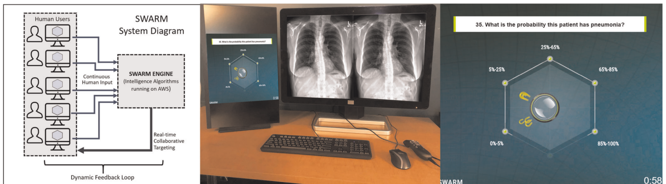
Fig. 7 Swarm platform. A system diagram (left image) of the Swarm platform shows the connection of networked human users. A Swarm engine algorithm received continuous input from the humans as they are making their decision and provides real-time collaborative feedback back to the humans to create a dynamic feedback loop. Swarm Platform positioned next to a second screen for viewing radiograph (middle image). A snapshot (right image) of the real-time swarm of six radiologists (group B) shows small magnets controlled by radiologists pulling on the circular puck in the process of collectively converging towards a probability of pneumonia. To view a video of the above question being answered in the Swarm platform, visit the following link: https://unanimous.ai/wp-content/uploads/2019/05/Radiology-Swarm.gif .
