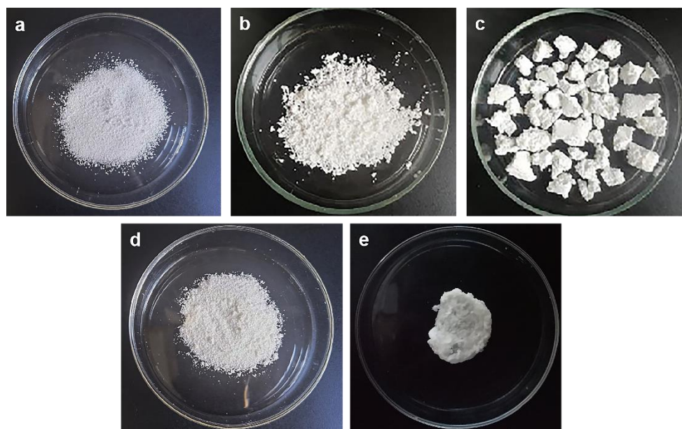
Figure 7. Photographs of polyethylenes obtained with ((a), S-C1-a 30 °C; (b), S-C1-a 50 °C; (c), S-C1-a 70 °C; (d), S-C1-b 30 °C; (e), homogeneous catalyst C1 30 °C).
