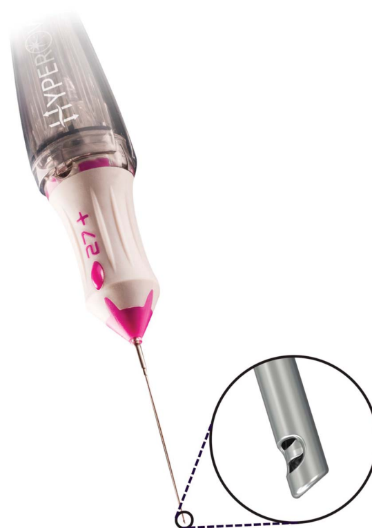
Fig. 1. HYPERVIT dual-cutting probe. Additional port in the internal cutter allows for cutting on both edges.
